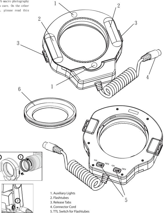
side of the front cover. If you push the switch down, the DMF880 flash unit will flash together with the macro flash to provide powerful lighting to your subject. It will be switched off if the switch is pushed up.
